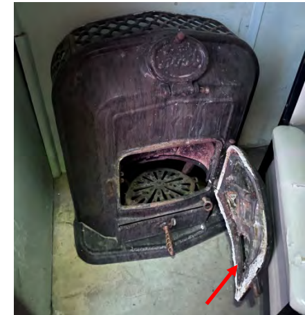
Photo 57: Dirty Linen – Friable asbestos fireplace rope
